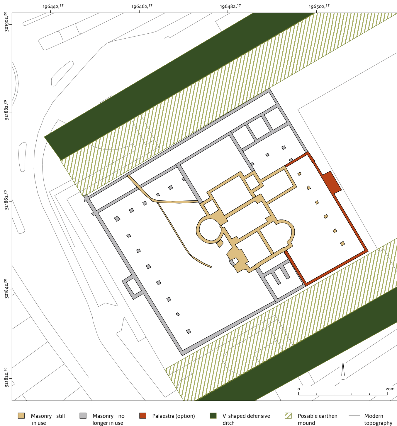
Figure 9.18 Reconstruction of the bathhouse in phase 4 showing, to the north and south, the ditch and the space between the wall and the ditch. The possible outdoor area at the bathhouse is reconstructed in red (showing part of the portico with eight footings) (source: K. Jeneson/M. Haars).
