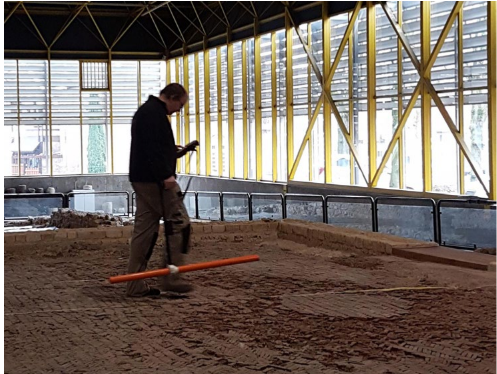
Figure 6.5 Electromagnetic survey being performed at the Roman Baths Museum (source: ArcheoPro, J. Orbons).
