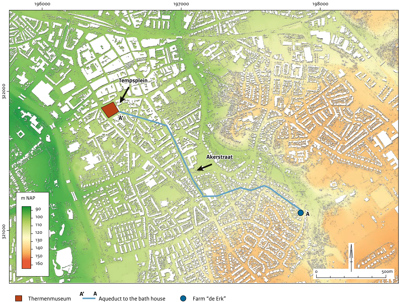
Figure 7.2 The reconstructed position of the proposed water supply to the baths complex on the elevation map, starting at De Erk farm (A) and ending at the Roman baths (A') (source: http://ahn.arcgisonline.nl/hoogteprofiel , M. Haars).
